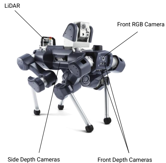
Fig. 5. ANYmal X (adapted from [14])
