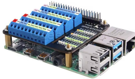
Fig. 24. Terminal Block for PPS Signal Distribution [18]
