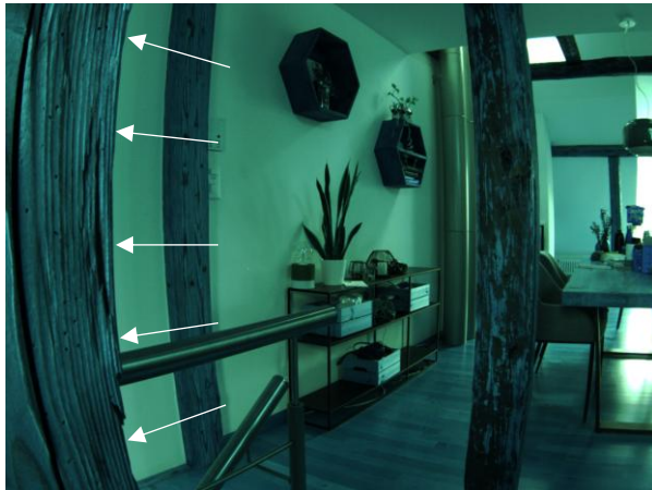
Fig. 37. Image With Distortion (Camera_2)
